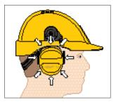
Low contact pressure is the best guarantee that hearing protectors are used. Two individually sprung headband wires of stainless spring steel provide an even distribution of pressure over the entire sealing ring. Eliminates the risk of point pressure and sound leakage, and provides a stable fit even during rapid head movements.
