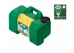
Model 7501 portable gravity operated eyewash shall include a FDA high-density green polyethylene 32l tank, ABS plastic eyewash heads with 1.5l/min flow rate over 15 minutes, yellow pull-down activation arm, integral handle on top, wide-fill threaded cap, label-mounted operating and maintenance instructions, stainless steel wall bracket (unit must be hung), and 1 bottle of bacteriostatic additive to permit storage of water for six months.
