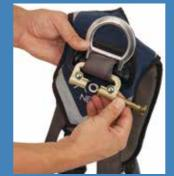
Slide connector through loosened web straps below back D-ring, then pull straps tight.
