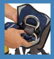
Open connector by pushing up plastic insert and karabiner gate inward. Insert nose of karabiner through swivel eye on SRL and rotate to the other side.
