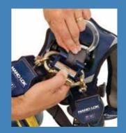
Close connector karabiner and rotate the plastic insert down to secure making sure the web straps pass through the slot on the insert.
