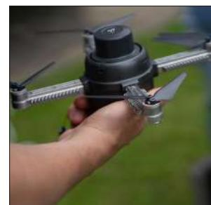
SKYLUX 200 is a modern lighting system integrated with a lightweight, tethered drone. It rises up to 12 meters and delivers 360° illumination with a 20,000-lumen light output. Ready for use in under 5 minutes—no masts or UAV permits required. Perfect for rescue missions, military operations, infrastructure inspections, and construction sites. Its tethered power supply allows continuous operation, and resistance to wind and rain ensures reliability in demanding field conditions.
